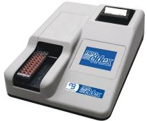
Ready-to-use ELISA instrument programmed with Monobind assays and proprietary formula designed, optimized and certified by Monobind for two-point analysis.
